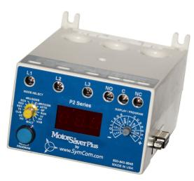
SymCom's Model 777-HRG-P2 is a fully programmable electronic overload relay that is designed for resistively grounded systems. The 777-HRG-P2 is recommended for monitoring and protecting any 3-phase 200-480VAC motor, used in a high resistance grounded (HRG) system, drawing 2-90 full load amps. The units provide unsurpassed protection from faulty voltage and current conditions.
